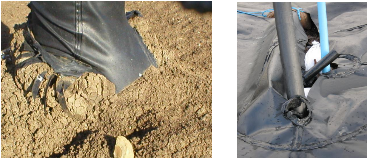
Figure 8.6: Damaged Boot Seals
