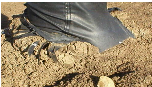
Damaged boot seal
